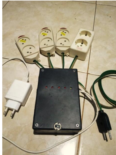
Figure 1. Prototype of IoT-Based Smart Home System with Voice Control
